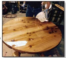
sections to flow into each other. Do not put layers on top of each other while they are still wet. This will produce uneven curing of the layers and cause ripples or "alligatoring" on the surface.
