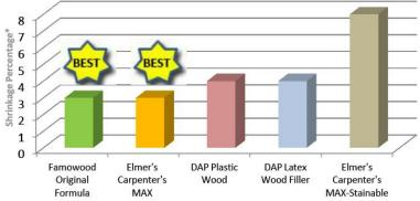
\*Volume was measured on a lab scale using the following formula: (Initial Volume - Final Volume) /Initial volume x 100 = Percent Shrinkage
